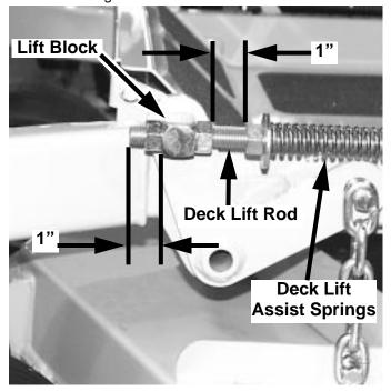
Left Rod Protruding Threads Figure 3-20
